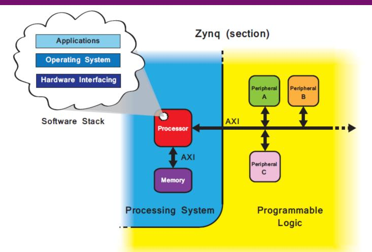
• **AXI** offers a means of **communication** between the processor and **IP blocks/cores** of an FPGA design.
